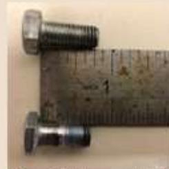
When this longer bolt is used, it presses against the starter shaft when tight and it messes up the Bendix operation.
