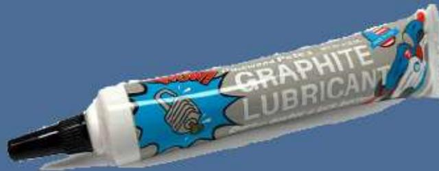
**YOU BUY THE GRAPHITE IN A SMALL TUBE WITH A POINTED TIP. YOU INSERT THE TIP INTO THE KEY HOLE AND "PUFF" SOME GRAPHITE INTO THE LOCK. THEN YOU INSERT AND REMOVE THE KEY SEVERAL TIMES TO WORK THE GRAPHITE INTO THE LOCK TUMBLERS, AND OPERATE THE LOCK A FEW TIMES.**
