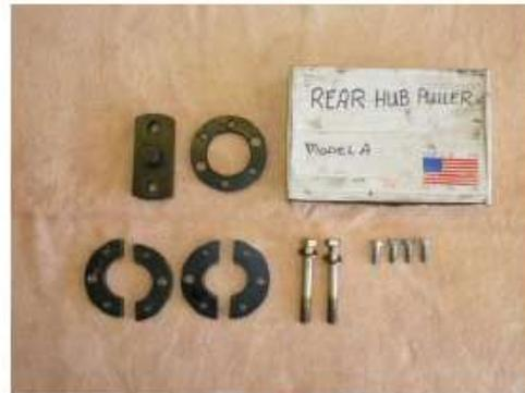
The Mitchell rear brake drum pulling tool: The two C-shaped parts (painted green on the left) are used to configure the tool to pull the shoulder and tapered design hubs. The two C-shaped parts (painted black on the right) are used to configure the tool to pull the grooved designed hubs.
