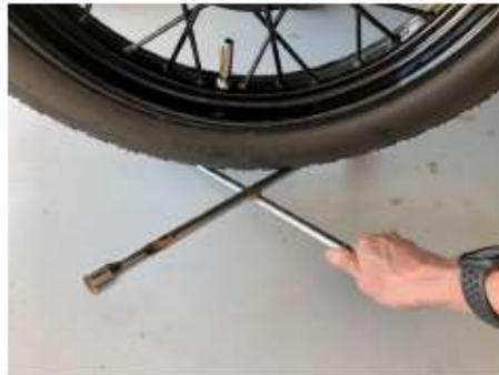
Hold the wheel in against the drum while you lower the lug wrench and use that free hand to start a lug nut on one of the studs. Once you have that lug nut started, you can let go of the wheel and start the rest of them. Use the tire iron to run them all in snug, then lower the jack and tighten them all again.
