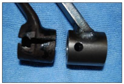
The crack propagates until there is not enough material to carry the load and it fractures when you depress the clutch pedal. The clutch pedal will not return, and you have lost your ability to disengage the clutch not fun when you are on tour a long way from home.
