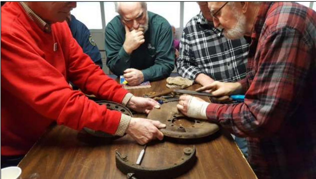
It was determined this unit had not been lubricated properly. It was also decided to use the next Tech Meet to assemble a Rear Backing Plate. Jim Hunter will be needing an assembly on his rebuild project.
