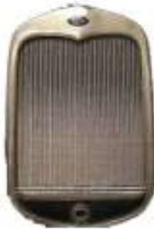
The Ford Service Bulletins of April, 1930 (page 450) advise that if you have excessive coolant loss though the radiator overflow tube, you can bend the tube back toward the back edge of the radiator filler neck. They also mention soldering in a brass washer where the tube passes through the baffle plate.
