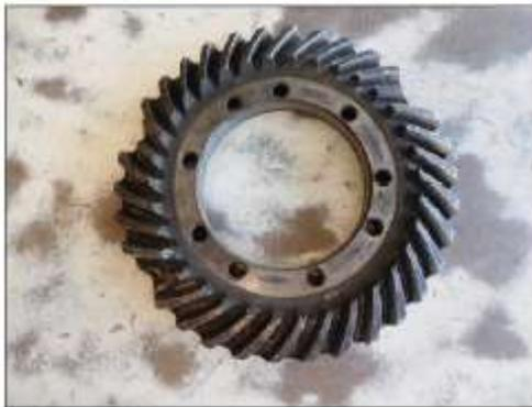
Teeth broken off the ring gear
